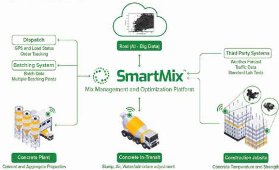
Fig. 10: A schematic of the SmartMix platform's interactions with data generated at the plant, in transit, and at the jobsite
