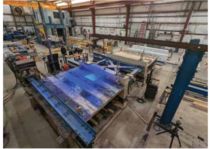
Large-scale tests demonstrated that externally bonded FRP retrofitting significantly improved both the shear strength and stiffness of deficient reinforced concrete diaphragms
