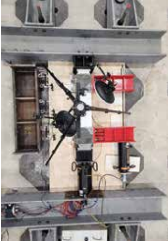
Test setup used to perform the flexural compression testing for the stress-strain analysis of BCSA cement specimens. The specimens were tested horizontally; all the gray steel pieces were attached to the strong floor to provide a reaction to the applied loads. For scale, the spacing of the octagonal steel plates in the floor is 4 ft (1.2 m)
